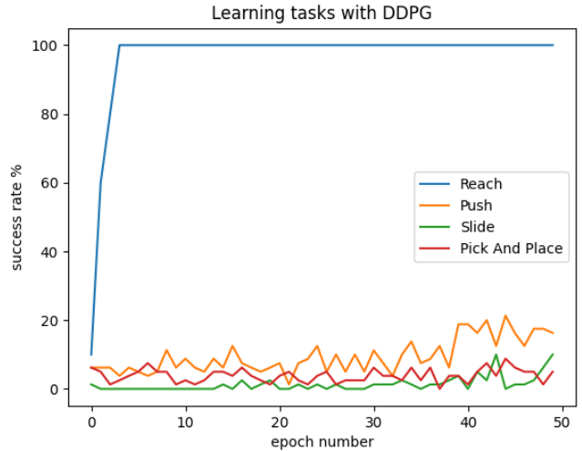
Fig. 6. How good agents learn in four given goal-oriented tasks. Except the FetchReach, the rest tasks are gradually learn something but in a very slow process. The success rate we are showing is tested in the evaluation.
